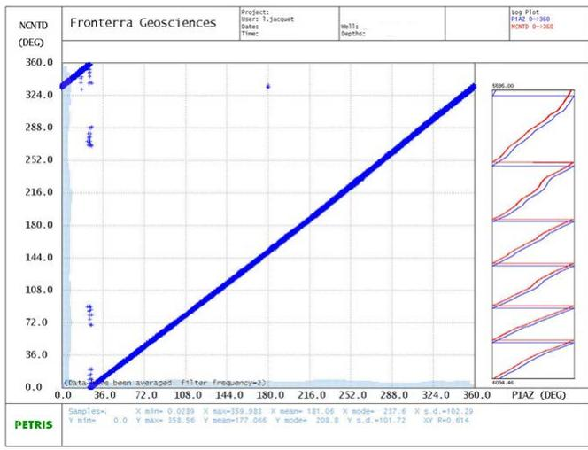
The example above is from an acoustic imaging tool, which has a set of magnetometers in the tool itself that can be used for orientation. However, the information from the orientation section is more typically used. A cross-plot of the “North” from the acoustic imaging tool against the equivalent curve from the orientation sonde should produce a straight line through the origin (0,0). In this case the orientation offset was incorrectly computed and
