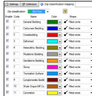
Task Fronterra's suggested dip vector symbol and color scheme for bedding and fractures in PETREL
